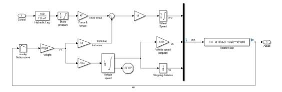
**Brake System Dynamics Subsystem**
