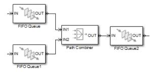
**Connecting a feedback path:** A feedback path enters the same queue as an ordinary path.
