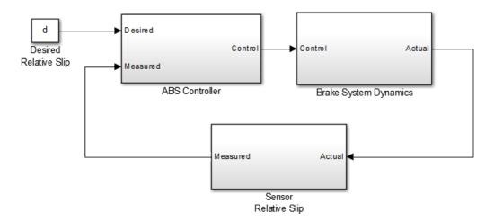
The model contains the following subsystem blocks that together form a completed closed-loop model of an ABS:
