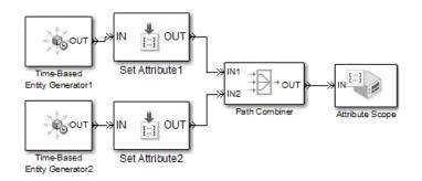
• **Merging queues:** Multiple queues merge into a single queue. (You might also use an Input Switch block for this, depending on the desired sequencing of entities in the single queue.)
