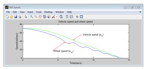
• The slip response of the braking system relative to the **Desired** setpoint. Throughout the simulation, the error between the desired slip value and the measured slip value remains small.
