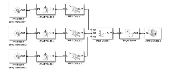
The three Set Attribute blocks assign a **Type** attribute to each entity, where the attribute value depends on which entity generator created the entity. FIFO Queue blocks store entities that cannot enter the Input Switch block yet because either
