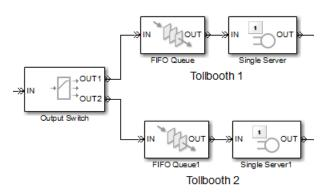
model below shows two queues in a parallel arrangement, preceded by a block that has one entity input port and two entity output ports.
