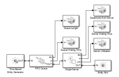
8 Run the simulation with different values of the **Period** parameter in the Time-Based Entity Generator block, as described in "Simulate with Different Intergeneration Times" on page 2-21. Look at the plots to see how they change if you set the intergeneration time to 0.3 or 1.1, for example.
