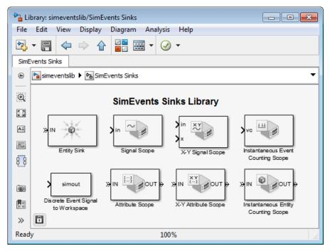
**8** Drag the Signal Scope block and the Entity Sink block from the library into the model window.
